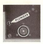
Winding the camera in reverse with either the single-frame shaft or the eight-frame shaft winds the motor. For multiple exposures, split frames, etc., it may be necessary to wind the film back more than one full run of the motor (about 35 feet).
