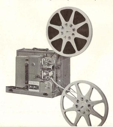
The Kodascope Royal Projector is designed to give the best in silent movie projection. It operates on both ac or dc, 105 to 125 volts, both forward and in reverse and has a speed control knob for rapid rewind.
