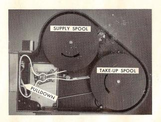
12 Attach the end of the film in the slot in an empty TAKE-UP SPOOL; then wind the film a few turns around the core, in the direction of the arrow, to take up the slack and to make certain that it is attached securely. The film must be attached so that the square hole in the spool will fit over the square base on the spindle.
