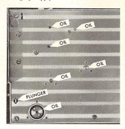
tached to the cork. Just touch the points indicated in the illustration so that a drop of oil runs down the sides of the shafts. After oiling, run the camera at normal (16) speed. Start and stop the camera several times to allow the oil to spread over the bearing surfaces. Wipe off the excess oil.
