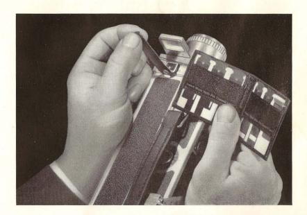
the subject you wish to record. For example, if the subject is on the left side (as viewed through the front finder), place the solid part of the mask on the left as it is inserted into the slot. When you are using the horizontal masks, use the mask with the solid part at the top for photographing subjects that appear at the top of the front finder.
